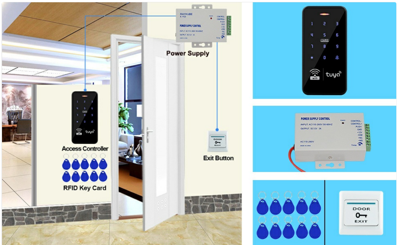
Figure 6: Wiring diagram showing connections between Access Controller, Power Supply, Exit Button, and Electric Locks (not included).
