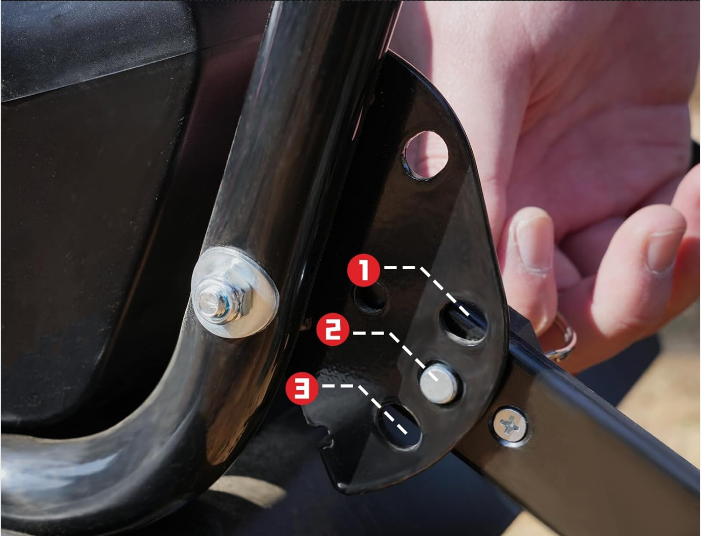
Image: A close-up view of the tiller's wheel height adjustment mechanism, showing three distinct positions for varying tilling depths or transport.
