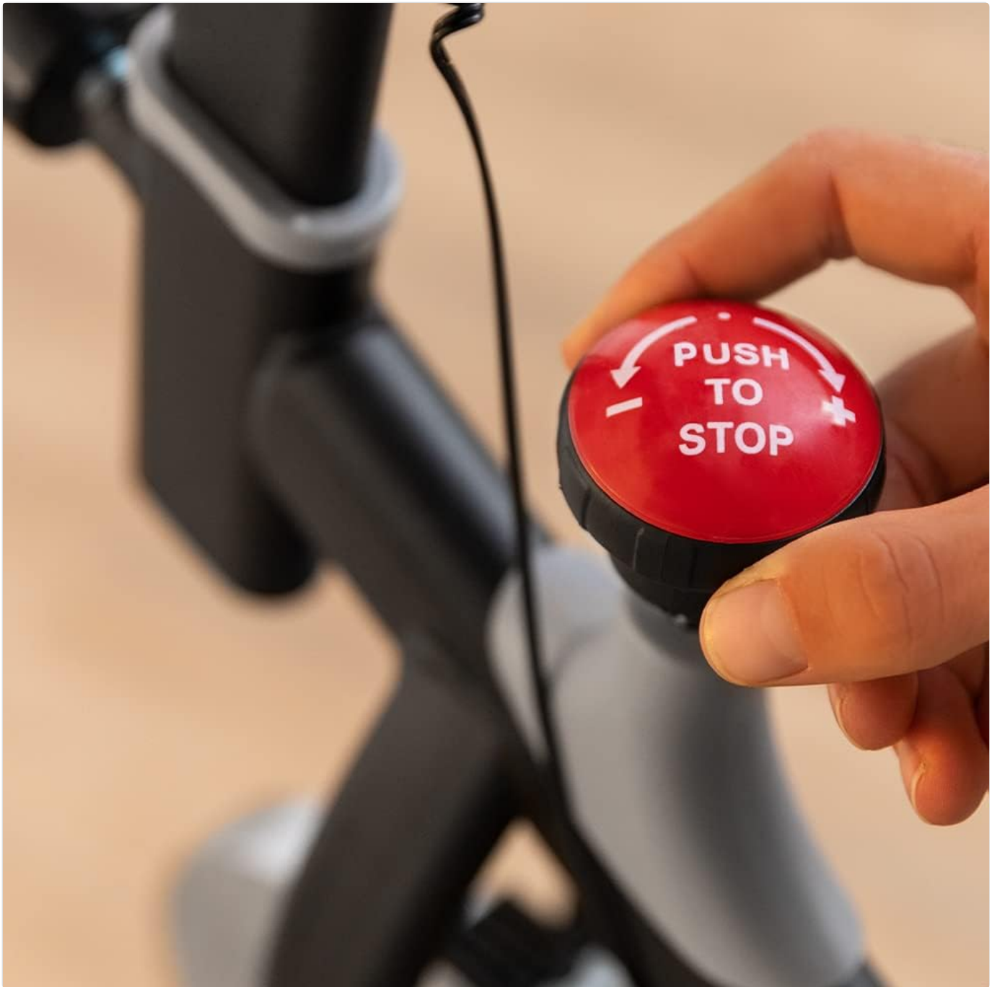
Image: A hand demonstrating the use of the red "PUSH TO STOP" emergency brake knob, located on the bike's frame.
