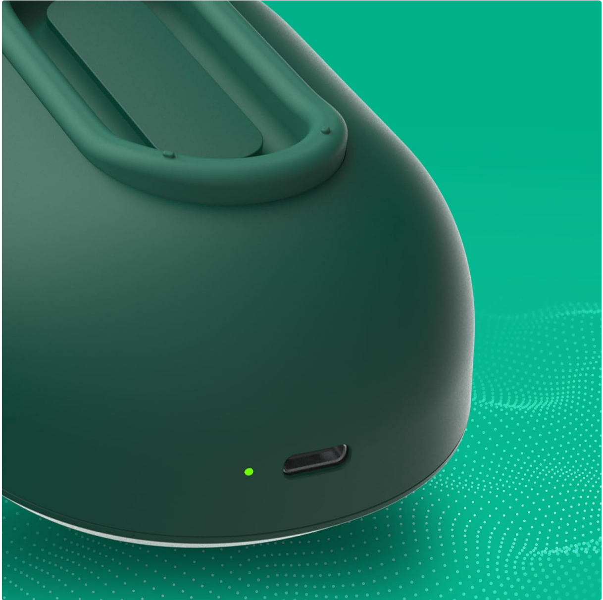
Image 3.1: The USB-C charging port located on the speaker, with a small green LED indicating power or charging status.
