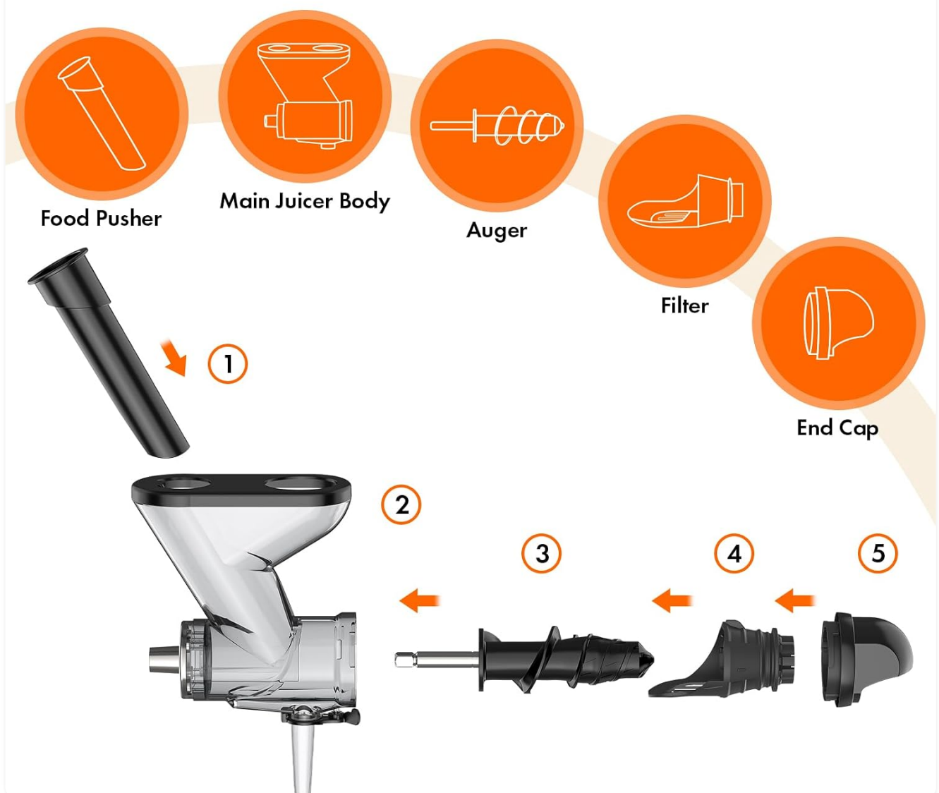
Figure 2: Exploded view of the juicer attachment components.
