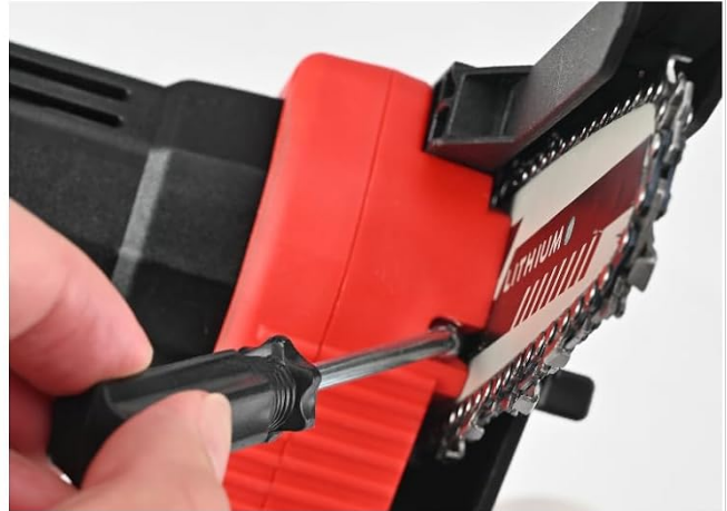
2. Tighten the screw and adjust the chain, expose 0.12inch when pulling down
