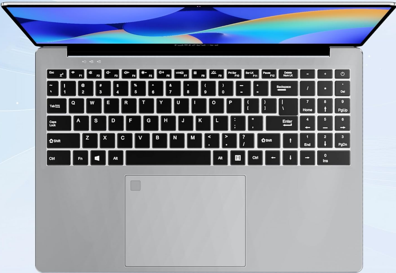
Image: Close-up view of the laptop's backlit keyboard, highlighting the numeric keypad, large touchpad, and fingerprint reader.
