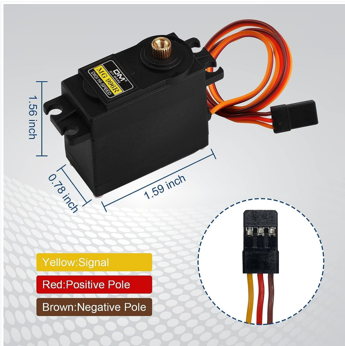
Image: MG996R servo dimensions and wiring color code: Yellow (Signal), Red (Positive), Brown (Negative).
