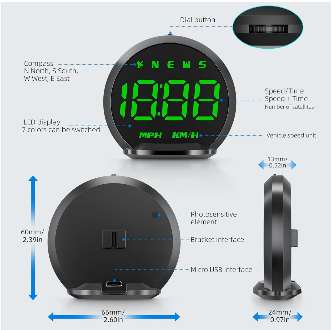
Image: A technical diagram of the G13 HUD, showing its dimensions (60mm height, 66mm width, 24mm depth) and labeling key components such as the dial button, compass display, LED display, photosensitive element, bracket interface, and Micro USB interface.
