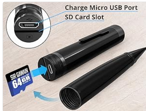
Image 5.1: Inserting the Micro SD card into the designated slot.
