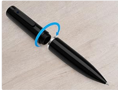
Image 5.2: Assembling the pen after inserting the Micro SD card.
