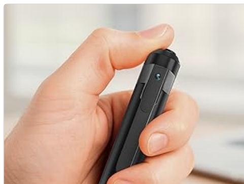
Image 6.1: The pen's operation is controlled by a single button.
