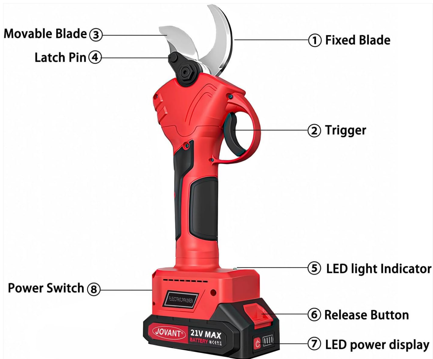
Figure 2.2.1: Labeled diagram of the JOVANT Electric Pruning Shears.
