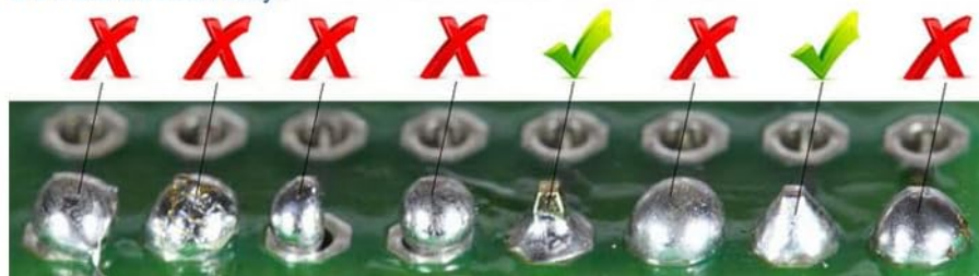
Figure 4.1.3: Illustration of soldering IC sockets, tact switches, and LEDs.
