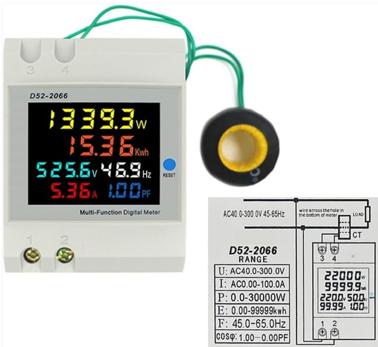
Image: The D52-2066 meter displayed alongside an external current transformer and a simplified wiring diagram. The diagram illustrates connecting the CT and voltage inputs to the meter.
