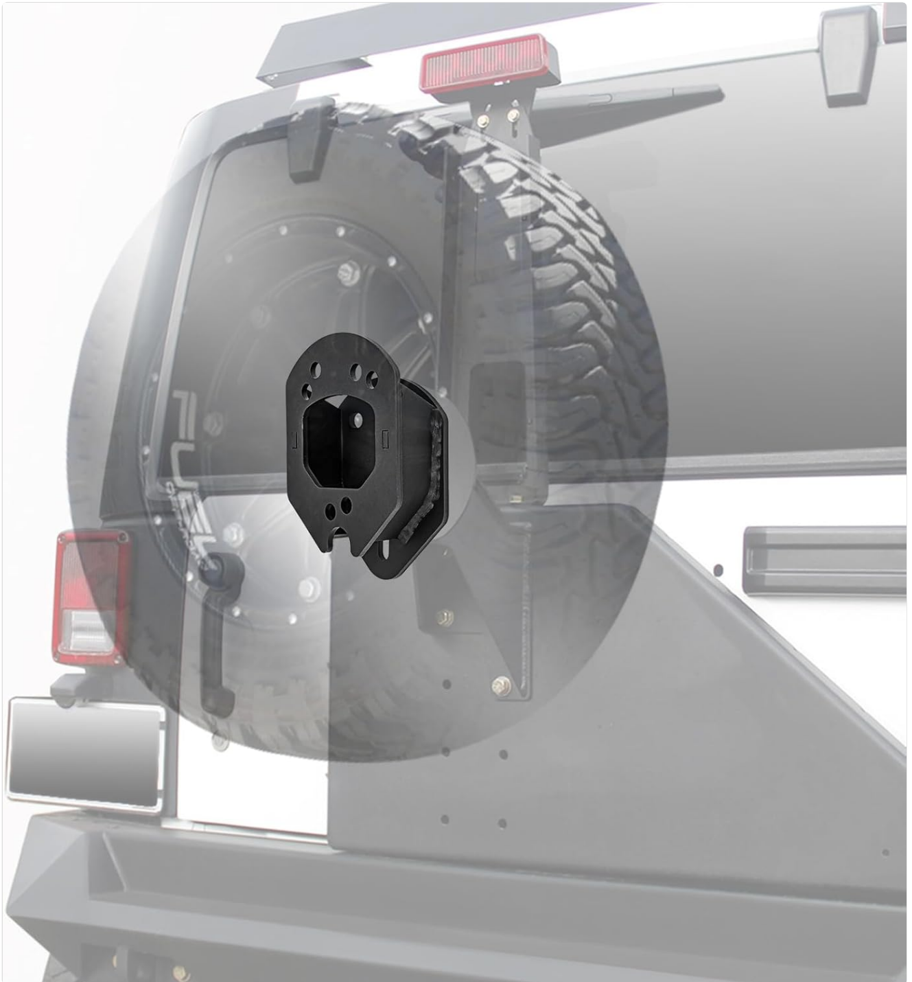
Image 4.1: The spacer block securely mounted to the vehicle's factory spare tire carrier, illustrating the initial installation step before
