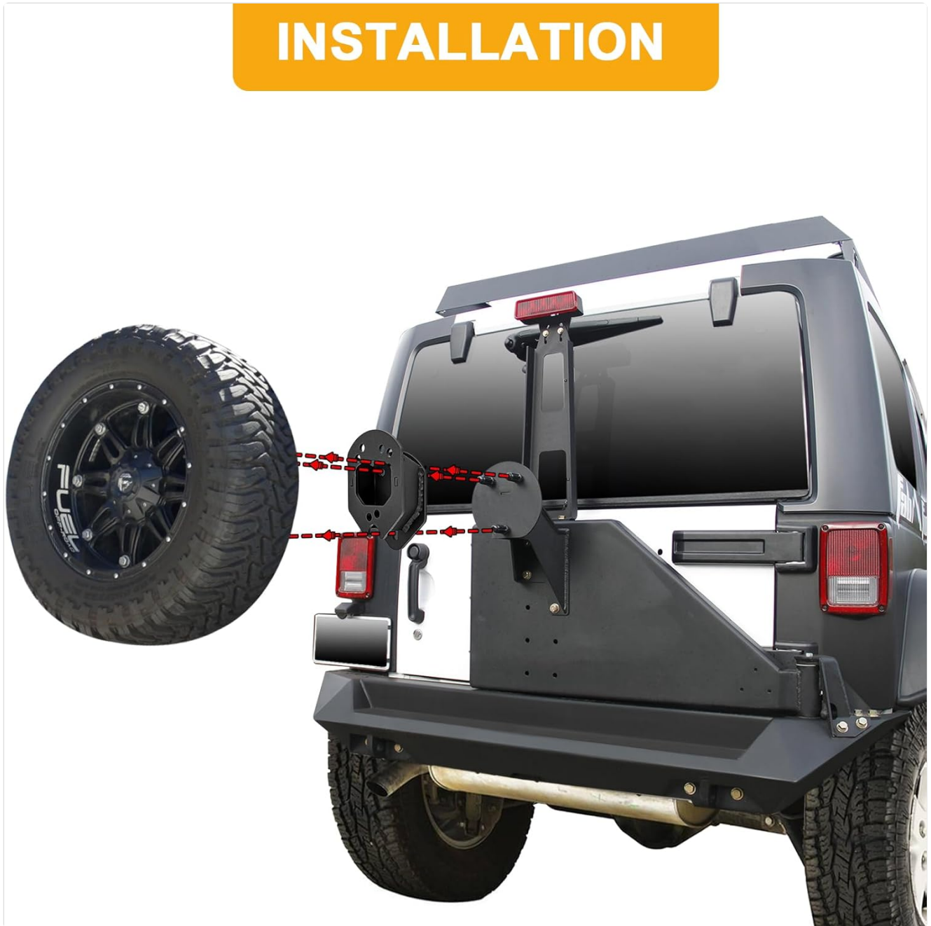
Image 4.2: An illustrative diagram demonstrating the placement of the spacer kit between the vehicle's spare tire mount and the spare tire itself, highlighting the outward and upward relocation.
