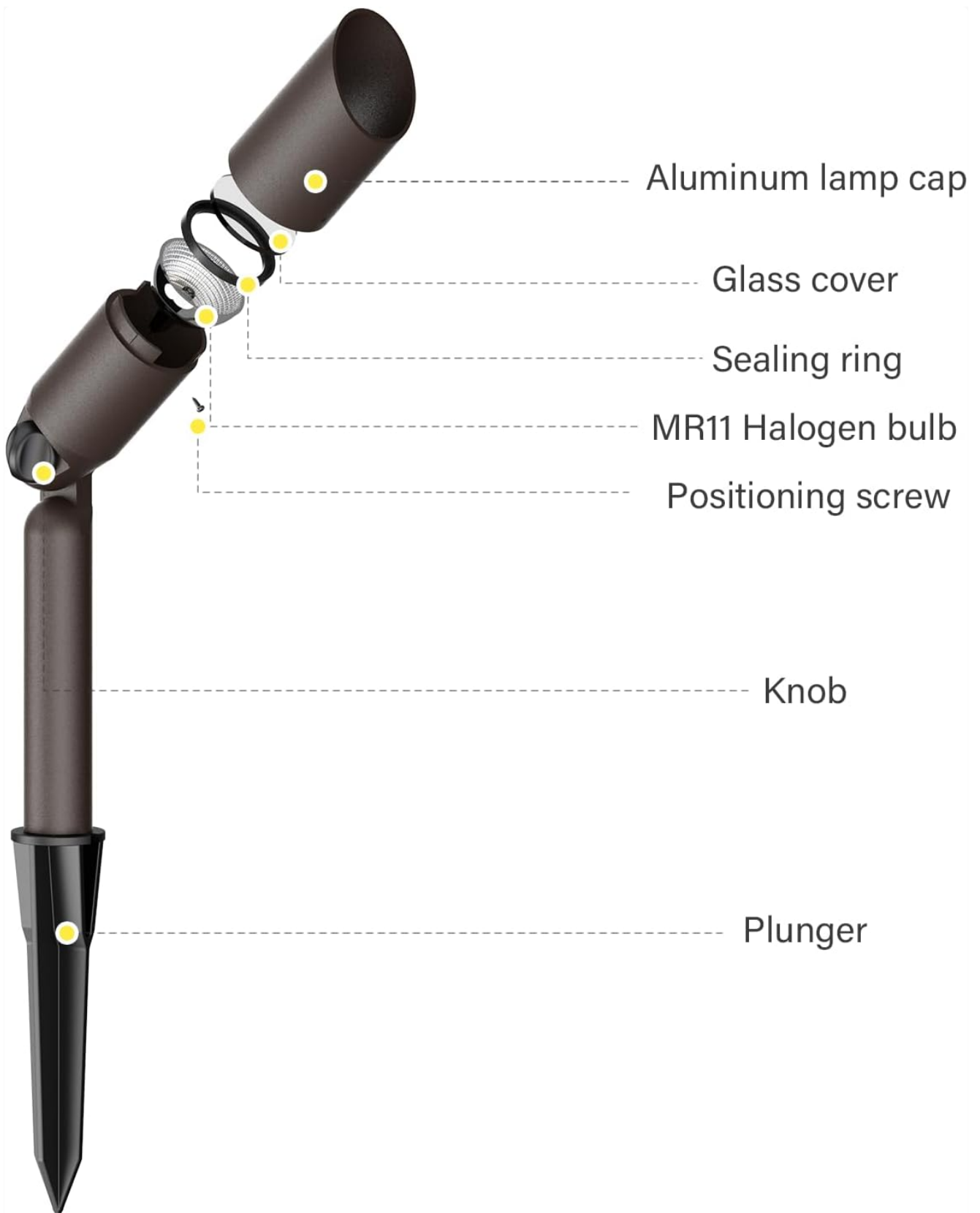
Figure 4.4: Exploded view of light components.
