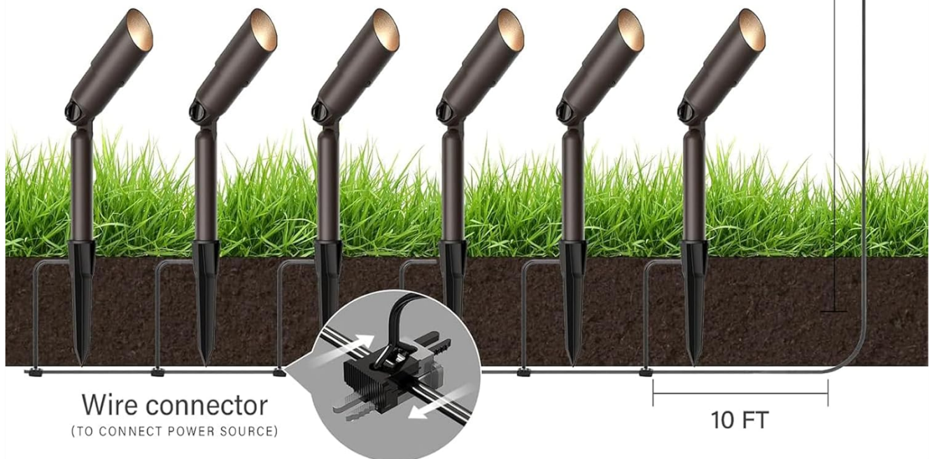
Figure 5.1: Installation procedure diagram.
