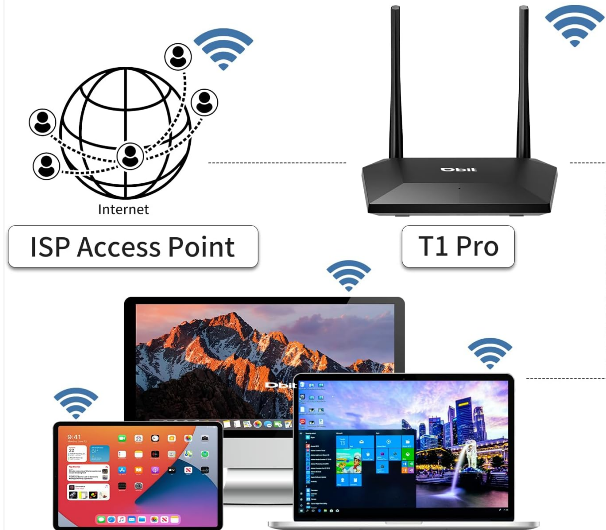
Image 5.1: A diagram showing the Wireless Repeater (WISP) function, where the T1 Pro router extends the network coverage from an ISP Access Point to multiple wireless devices.
