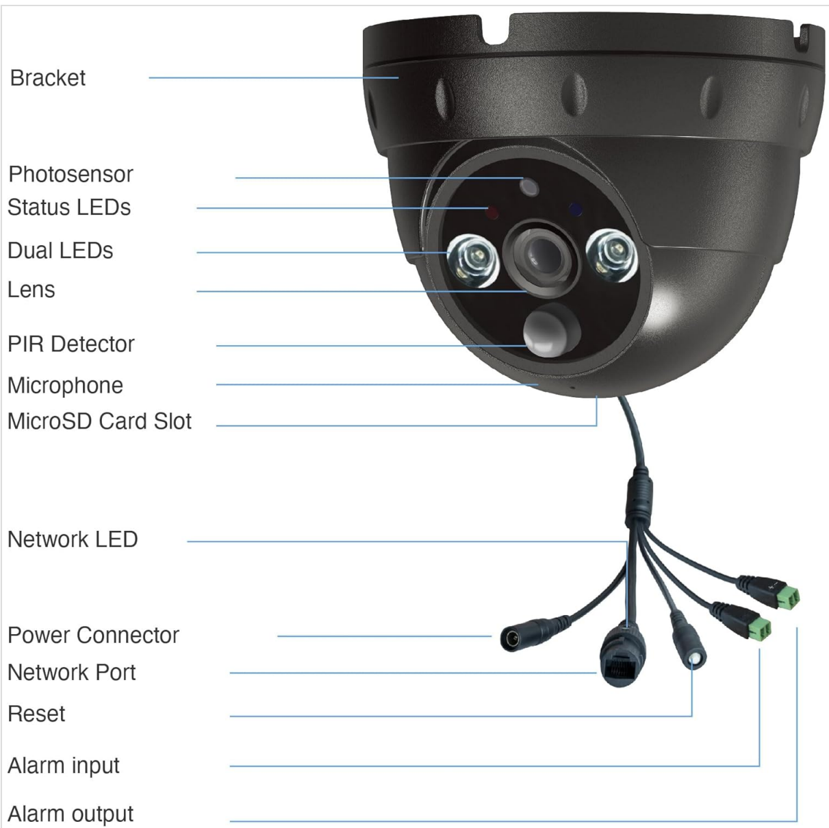
Image Description: A detailed diagram of the INSTAR IN-8403 camera, highlighting its key components. These include the bracket for mounting, photosensor, status LEDs, dual LEDs for illumination, the main lens, PIR detector, microphone, and MicroSD card slot. The diagram also shows the cable connections for the network LED, power connector, network port, reset button, alarm input, and alarm output.
