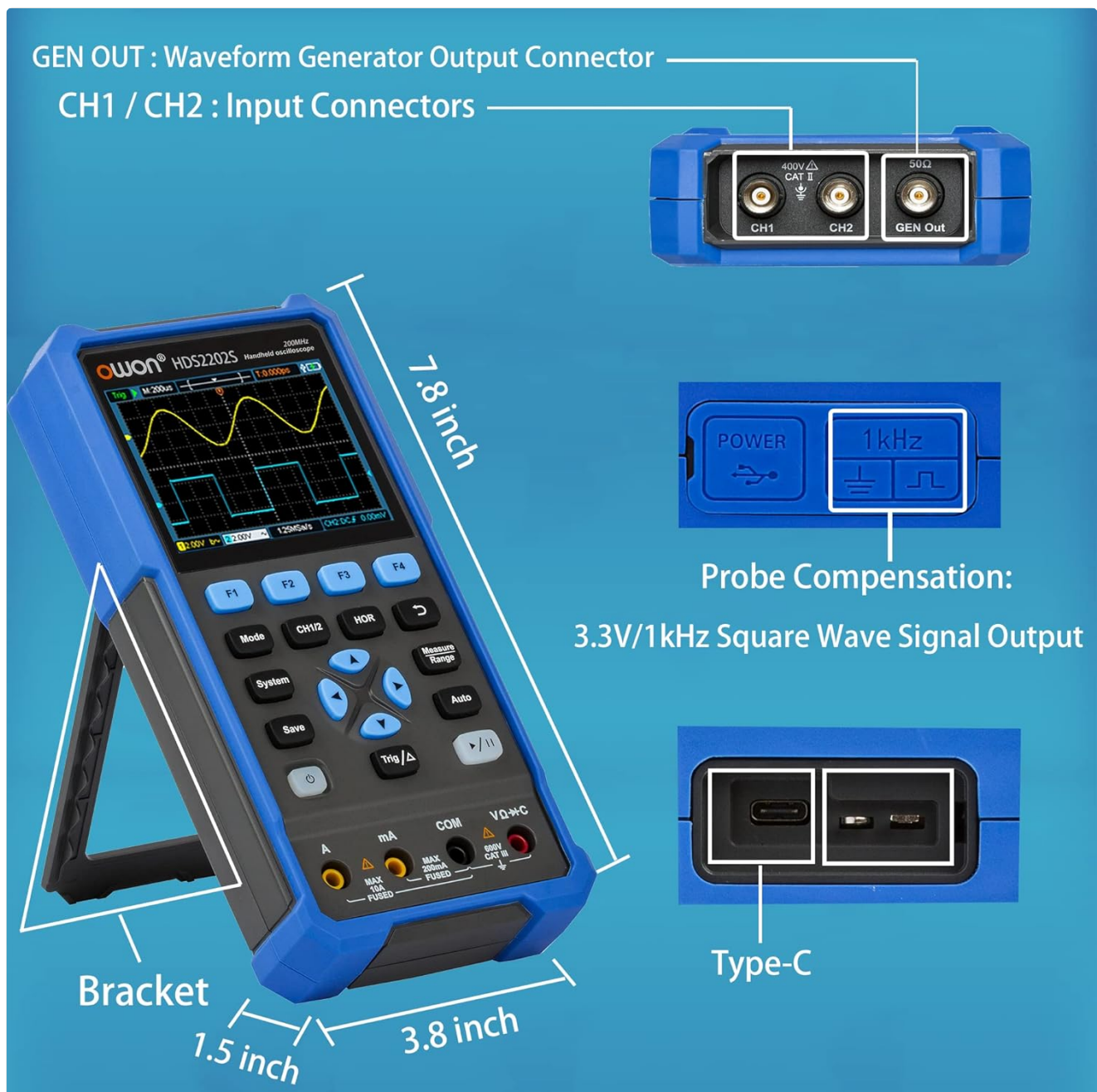
Figure 6: HDS2202S port locations and dimensions.
