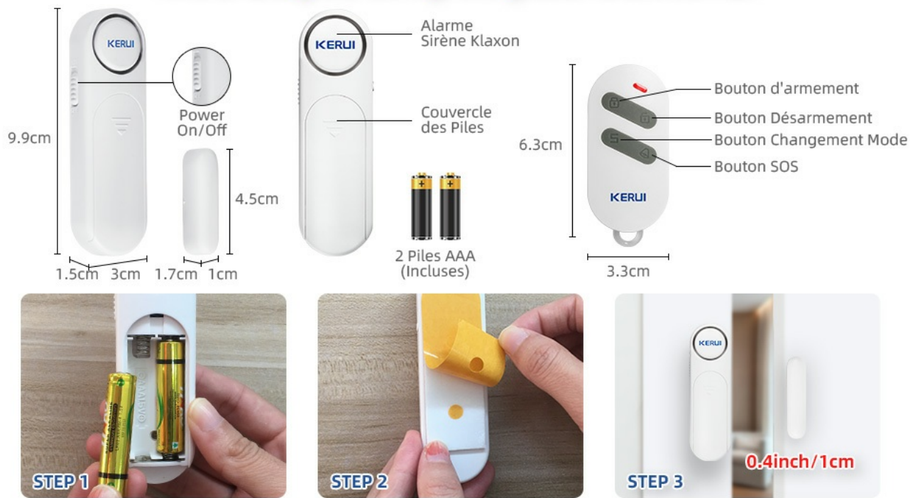
Image 4.1: Simple Installation Steps for the KERUI Alarm. Step 1: Insert 2 AAA batteries into the main alarm unit. Step 2: Peel off the protective film from the adhesive patch and attach it to the back of the main alarm unit and the magnetic strip. Step 3: Mount the main unit and magnetic strip on the door/window frame, ensuring they are aligned and separated by no more than 1 cm (0.4 inches) when the door/window is closed.
