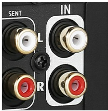
Image: Close-up view of the RCA input ports (IN) on the rear panel.
