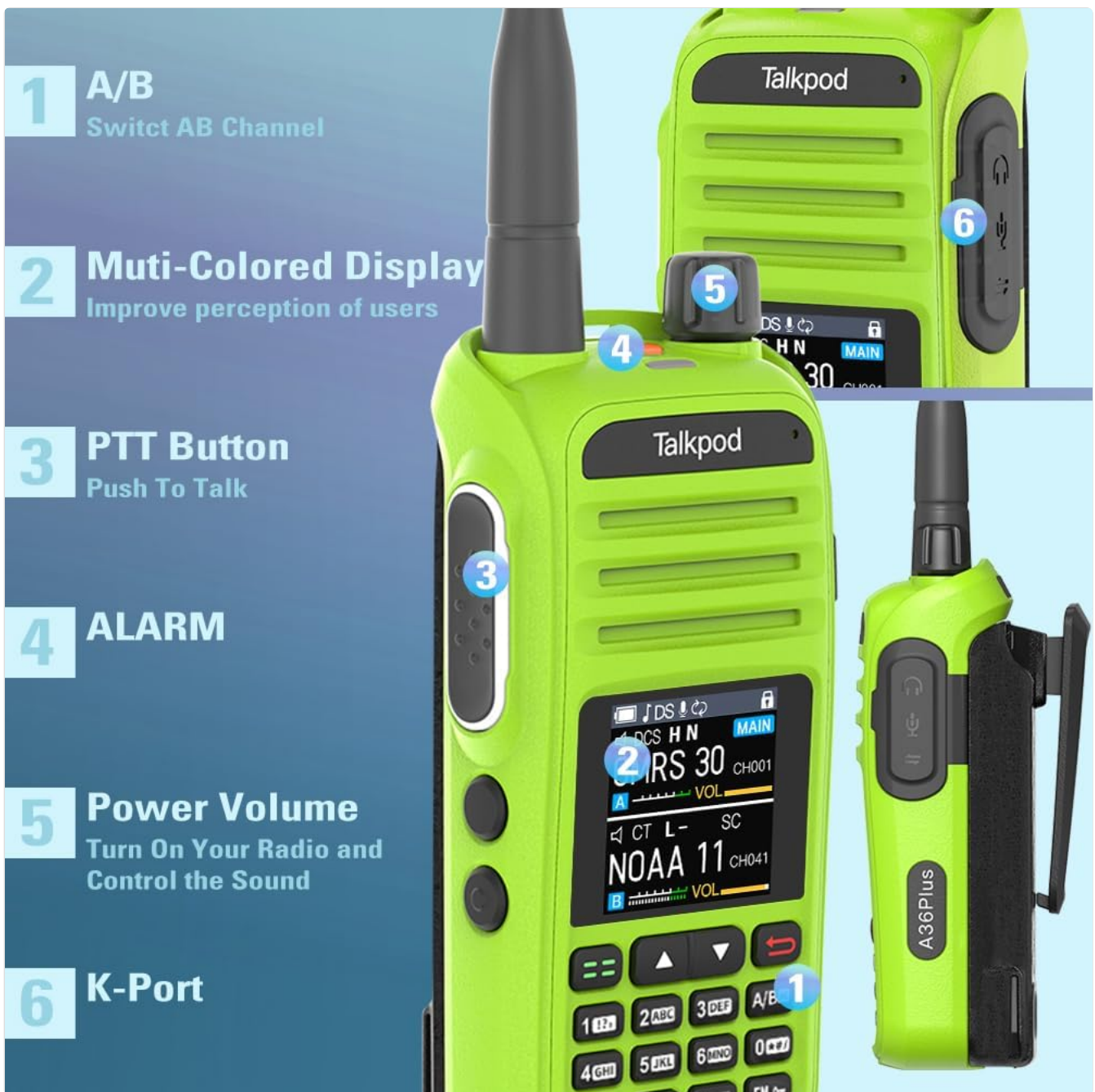
Figure 2.4: Labeled diagram of the Talkpod A36Plus, pointing out key components such as the A/B switch, multi-colored display, PTT button, alarm button, power/volume knob, and K-Port.
