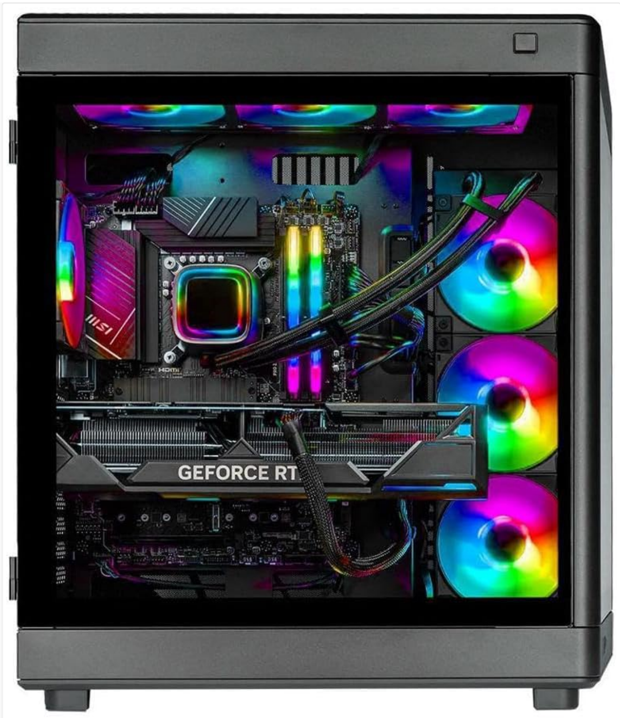
Figure 4.2: A detailed view of the NVIDIA Geforce RTX 4090 graphics card installed within the system.
