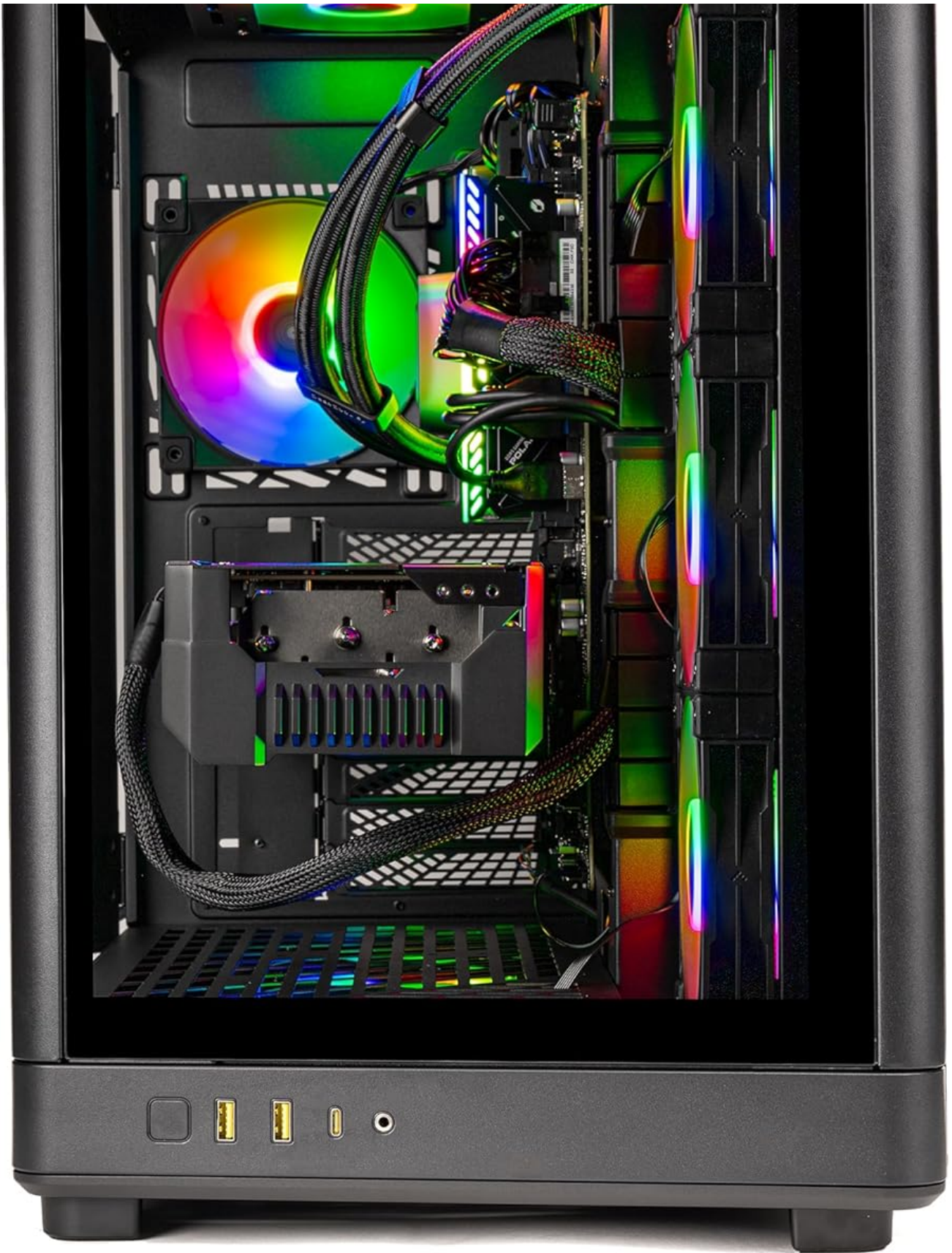
Figure 3.3: Close-up of the top front panel, highlighting the power button, reset button, USB 3.0, USB-C Gen 2, and headphone/mic inputs.
