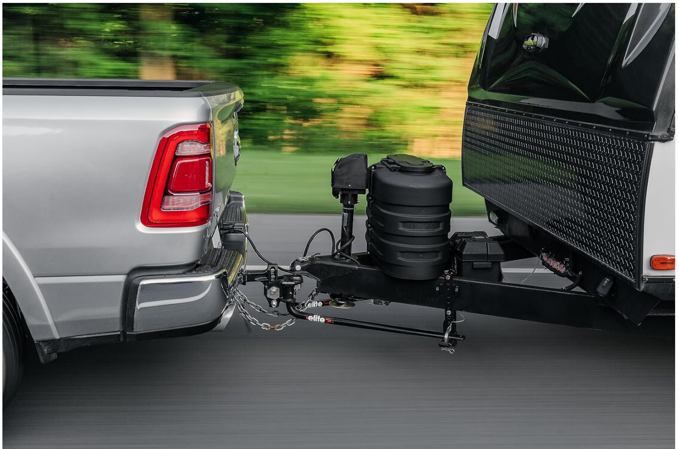
Image: A complete view of the Camco Eaz Lift Elite-S weight distribution hitch installed, connecting a tow vehicle to a trailer, demonstrating the system in use.
