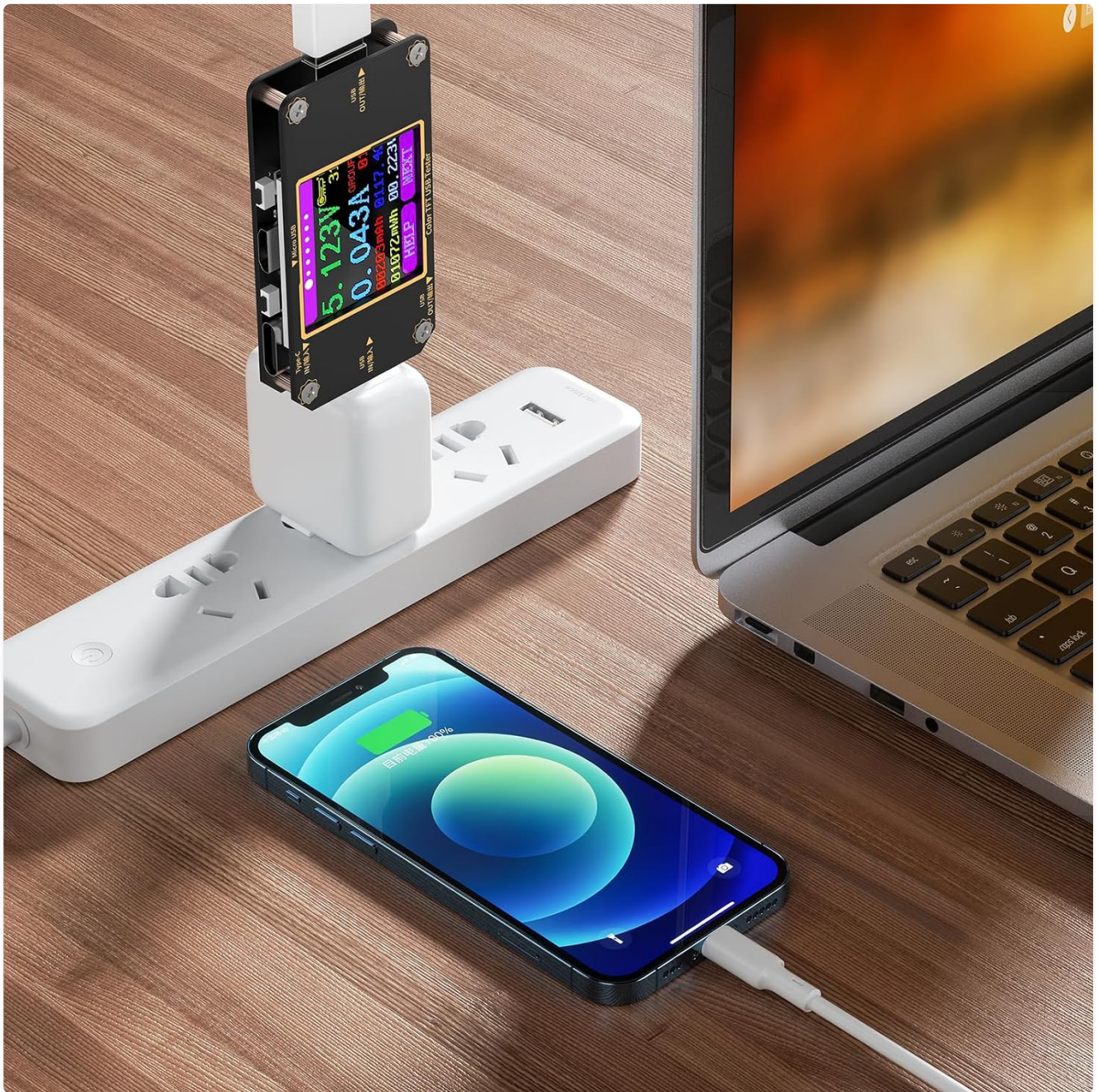
Figure 8: The USB Tester Meter A3 in use, measuring the charging performance of a smartphone connected to a wall charger.
