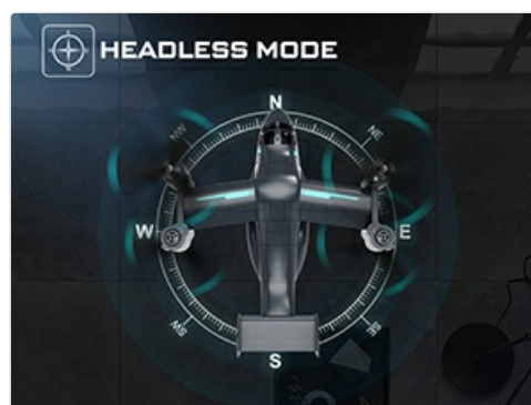
Image: An illustration of Headless Mode, showing how the drone's direction is relative to the controller.
