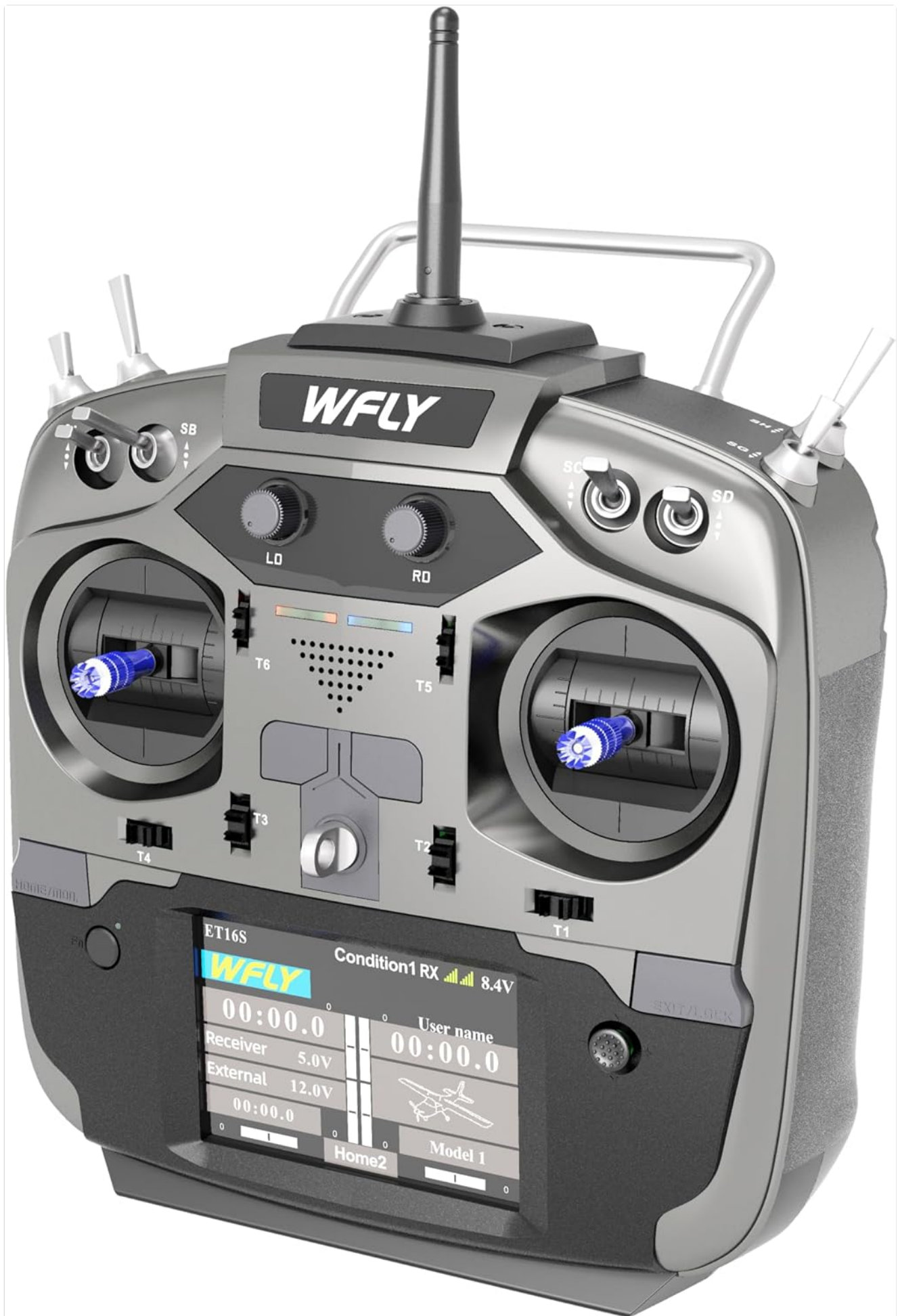
An angled view of the WFLY ET16S transmitter, showcasing its ergonomic design, the central touch screen, and the various switches and gimbals.
