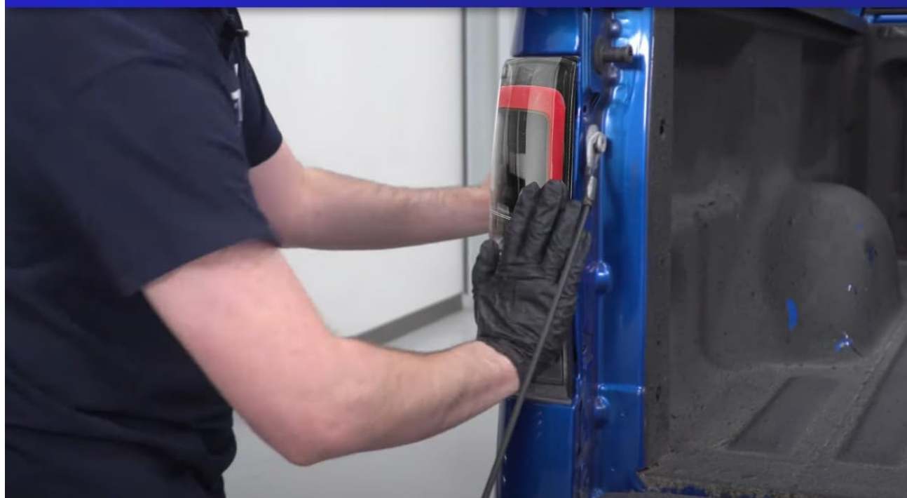
Image: Demonstrating the easy installation process of the tail light.
