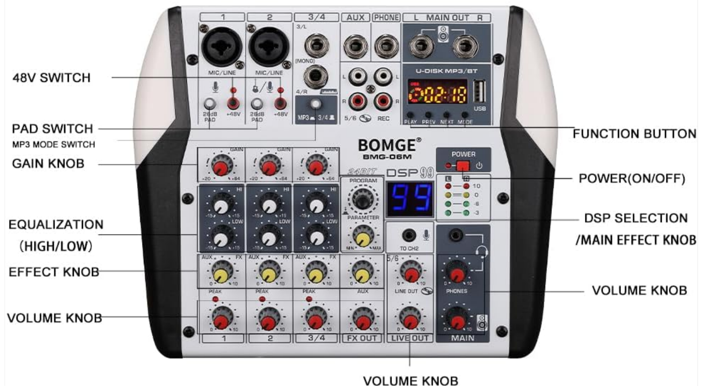
Figure 2: Front Panel Controls and Functions
