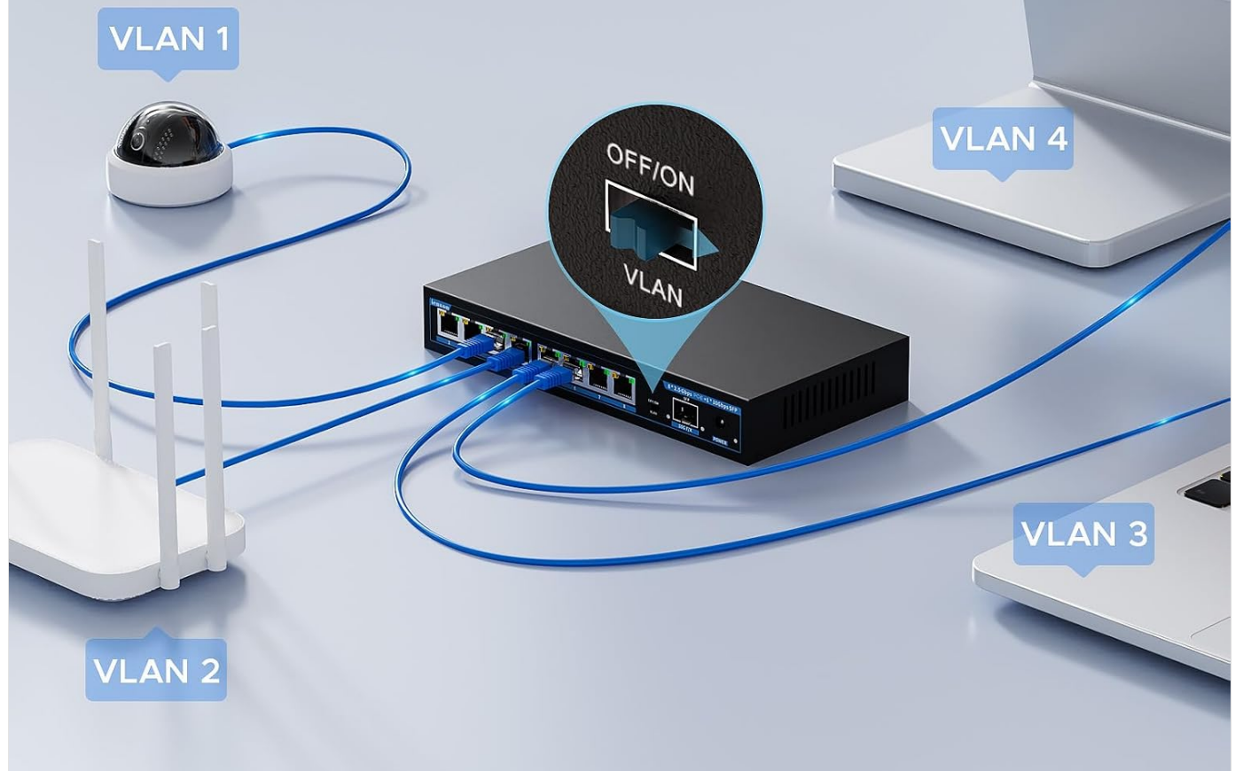
Figure 5.2: Illustration of VLAN mode for enhanced security.
