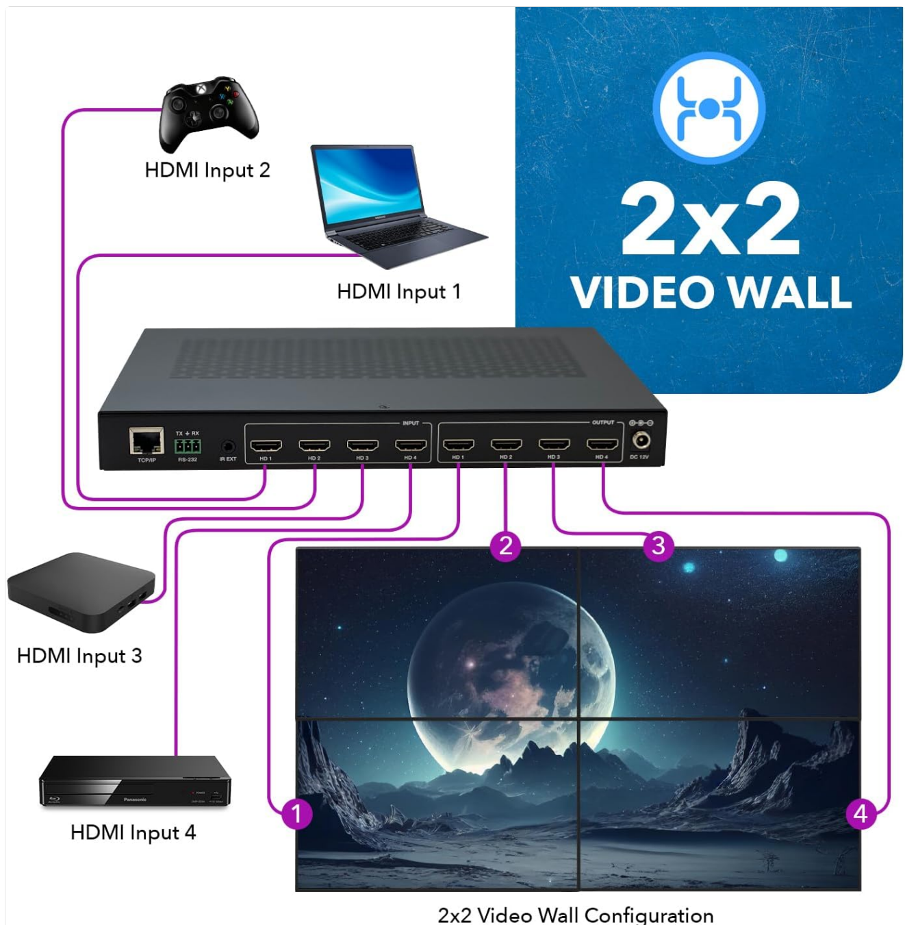
Image 5.2: Example of a 2x2 Video Wall Configuration, demonstrating how a single HDMI input source can be expanded and displayed across four synchronized screens to form one large image.
