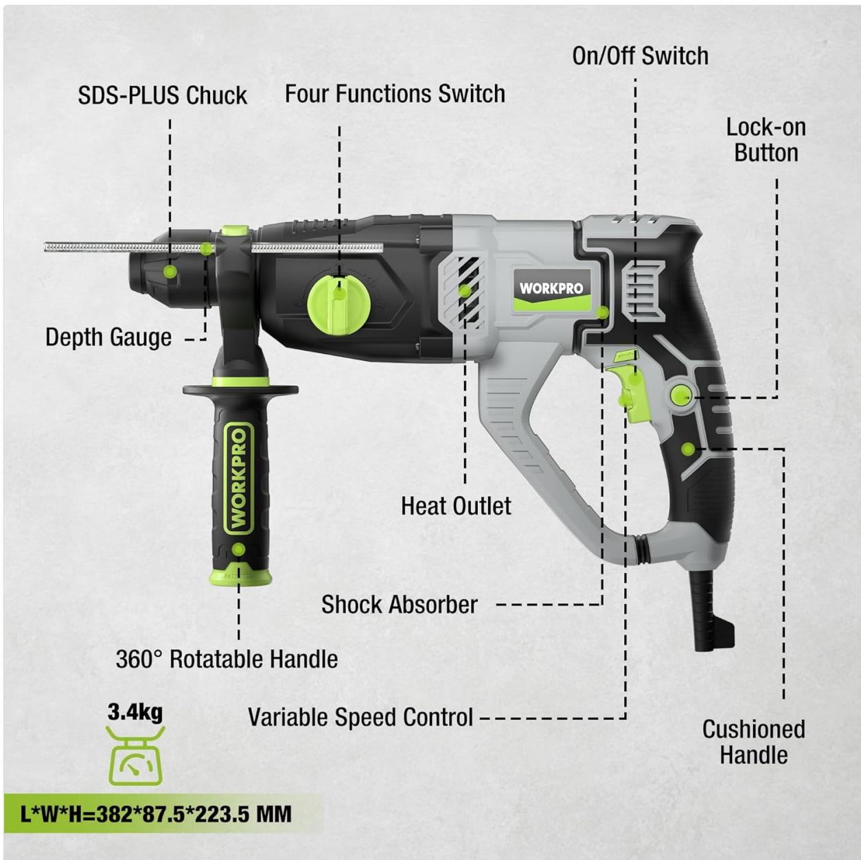
**Image Description:** A detailed diagram labeling key components of the rotary hammer drill: SDS-PLUS Chuck, Four Functions Switch, On/Off Switch, Lock-on Button, Heat Outlet, Shock Absorber, Variable Speed Control, Cushioned Handle, 360° Rotatable Handle, and Depth Gauge.
