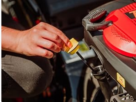
Image 2.3.1: A hand carefully pouring engine oil into the oil fill opening of the lawn mower. This step is essential before the first use to ensure proper engine lubrication.
