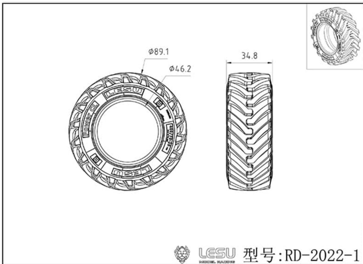
Figure 7.1: Technical diagram with key dimensions of the LESU RD-2022 tyre.
