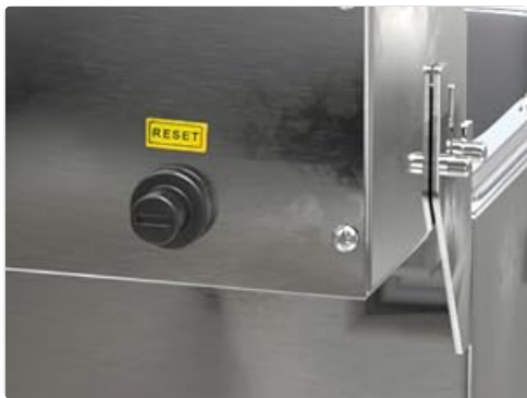
Image: A close-up of the reset button, which may need to be pressed if the fryer does not power on or heat correctly.
