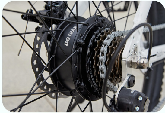
Figure 5.3: The 7-speed gear system for versatile riding.
