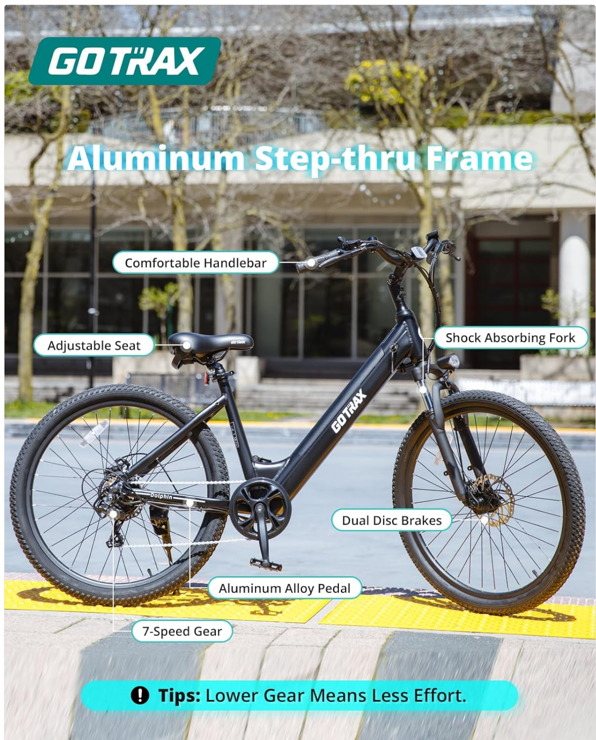
Figure 4.1: Key components of the Gotrax Dolphin Electric Bike.
