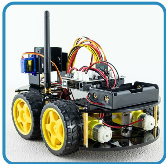
Image: The LAFVIN LA044 Robot Car Kit viewed from multiple angles, showcasing its chassis, wheels, sensors, and main control board.
