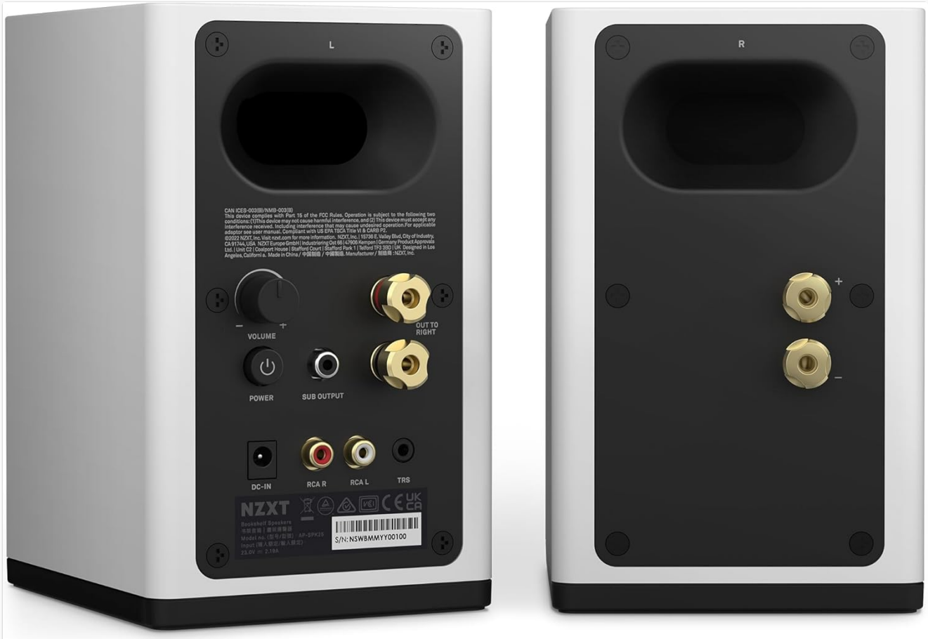
Figure 3.1: Rear panel connections including DC-IN, RCA, TRS, and speaker terminals.
