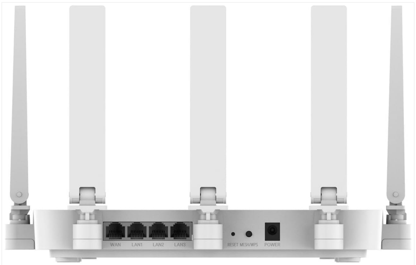
Figure 4.3: Rear view of the ZTE E1320 Router, showing WAN, LAN ports, Reset/WPS button, and Power input.
