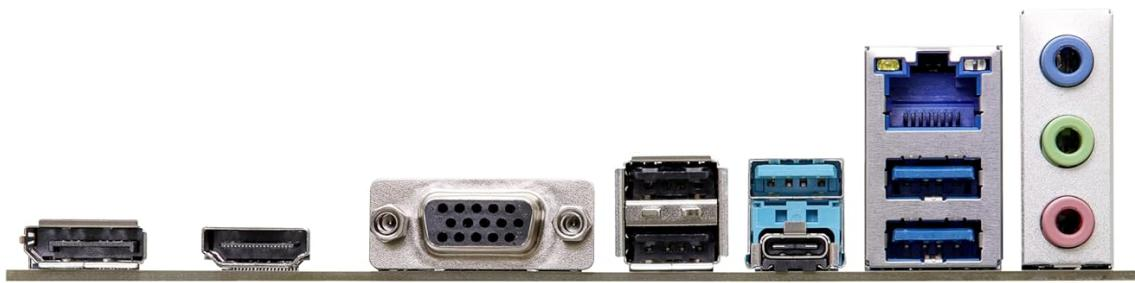
Figure 3.2: Rear I/O panel of the ASRock B760M-HDV/M.2 Motherboard, showing USB ports, display outputs (HDMI, DisplayPort, D-Sub), and audio jacks.
