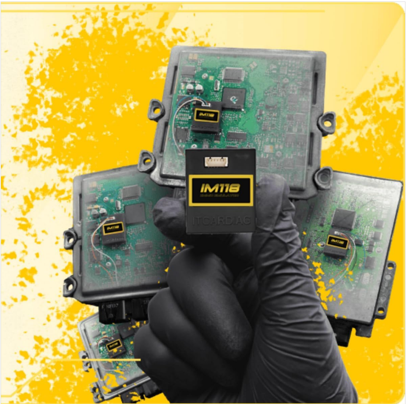
Image: A gloved hand holding the ITCARDIAG IM118 IMMO Emulator module above several vehicle Electronic Control Units (ECUs), illustrating its application in ECU work.
