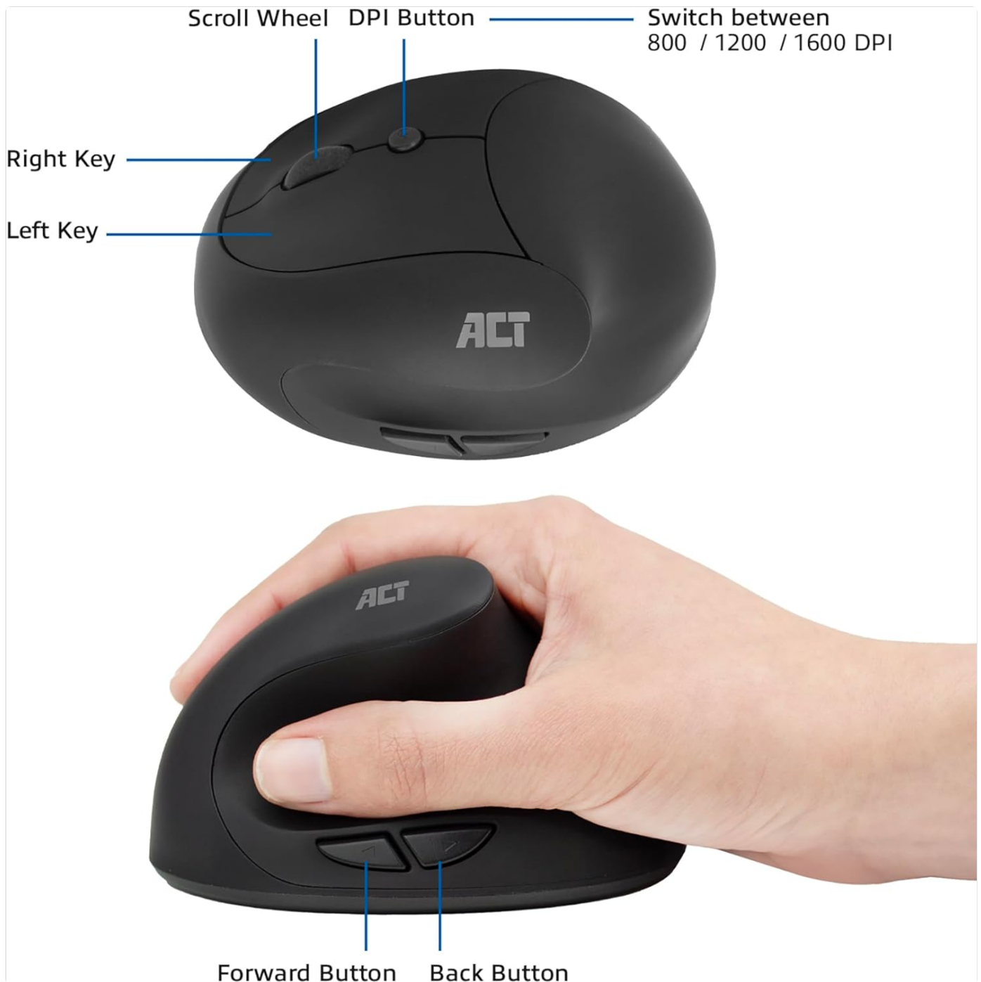
Image 3.1: Diagram showing the buttons on the ACT AC5101 mouse. These include the Left Key, Right Key, Scroll Wheel, DPI Button, Forward Button, and Back Button.
