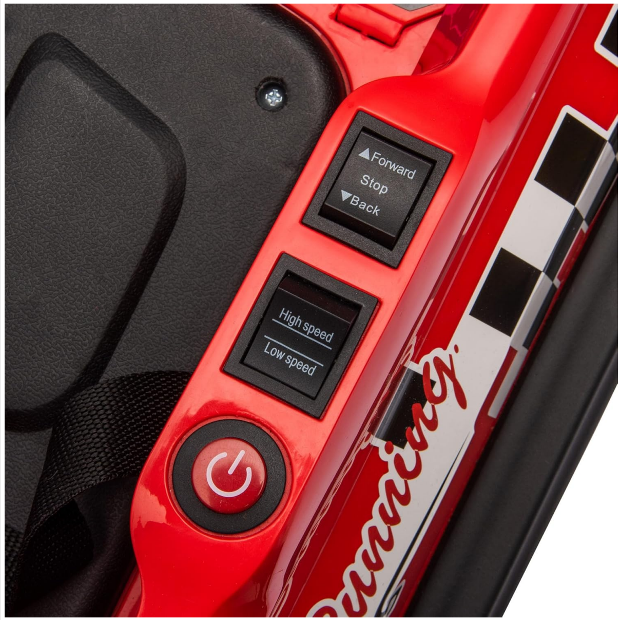
Figure 3.1: Control panel with power button and speed/direction switches. The charging port is typically located near these controls or under the seat.
