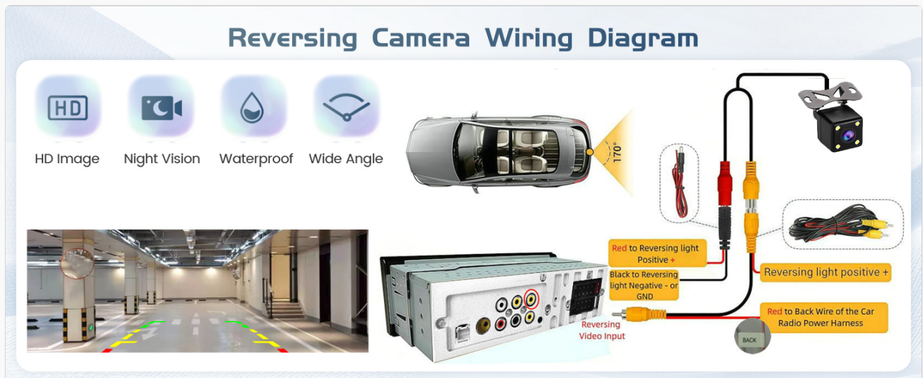
Image 2.3: Reversing Camera Wiring Diagram. This diagram illustrates the connections for the included backup camera, showing how to connect it to the vehicle's reverse lights and the head unit's video input.
