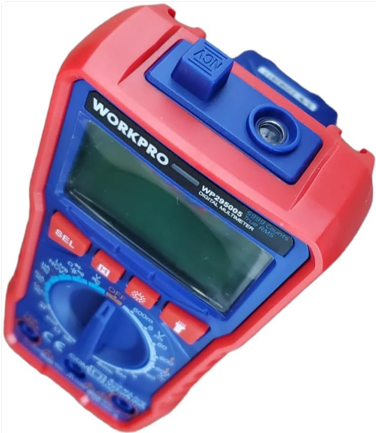
Figure 2: Top view of the multimeter, highlighting the NCV (Non-Contact Voltage) sensor.
