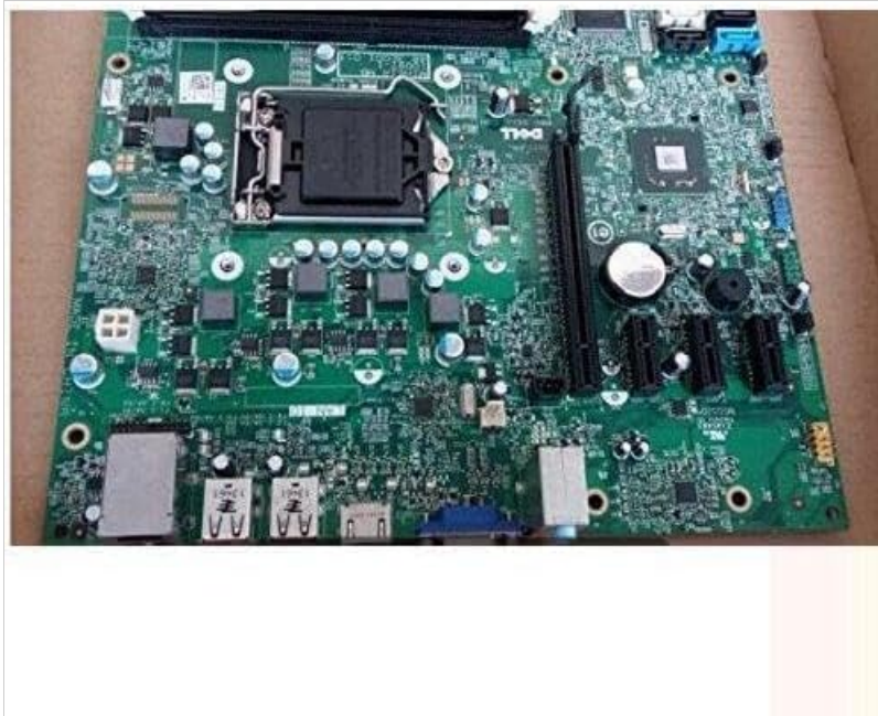
Image 1: Top-down view of the Generic M5DCD Optiplex 390 Motherboard Systemboard, showing the CPU socket, RAM slots, PCIe slots, SATA ports, and various I/O connectors.
