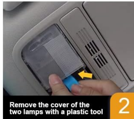
Image: Installation steps for overhead console removal.
