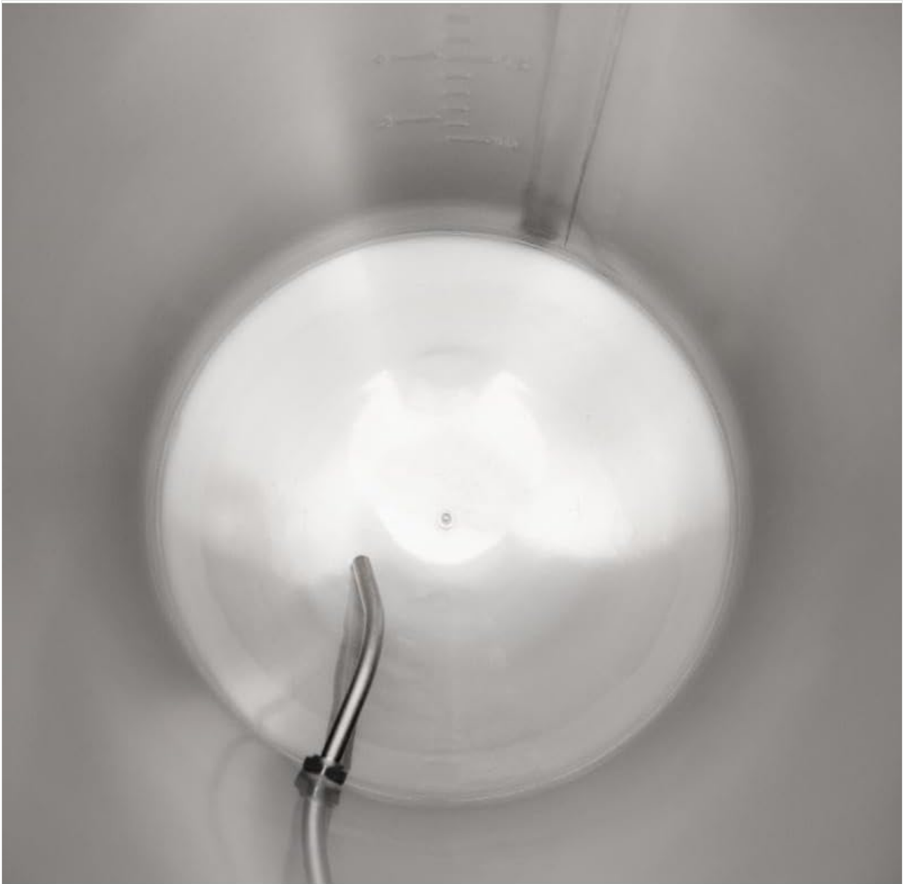
Figure 3.9: Internal view of the fermenter. This image clearly shows the domed base for complete drainage and the rotating rack arm positioned near the outlet.
