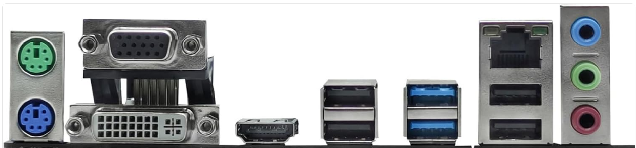
Figure 3.2: Rear I/O panel showing PS/2 ports for keyboard and mouse, VGA port, DVI port, HDMI compatible port, USB 2.0 ports, USB 3.0 ports, RJ45 LAN port, and audio jacks.
