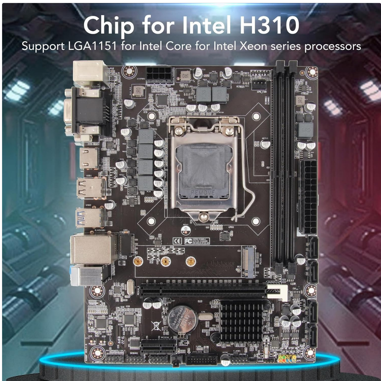
Figure 2.1: Top-down view of the Dpofirs H310 LGA 1151 Micro ATX Motherboard, highlighting the CPU socket, RAM slots, and various connectors.
