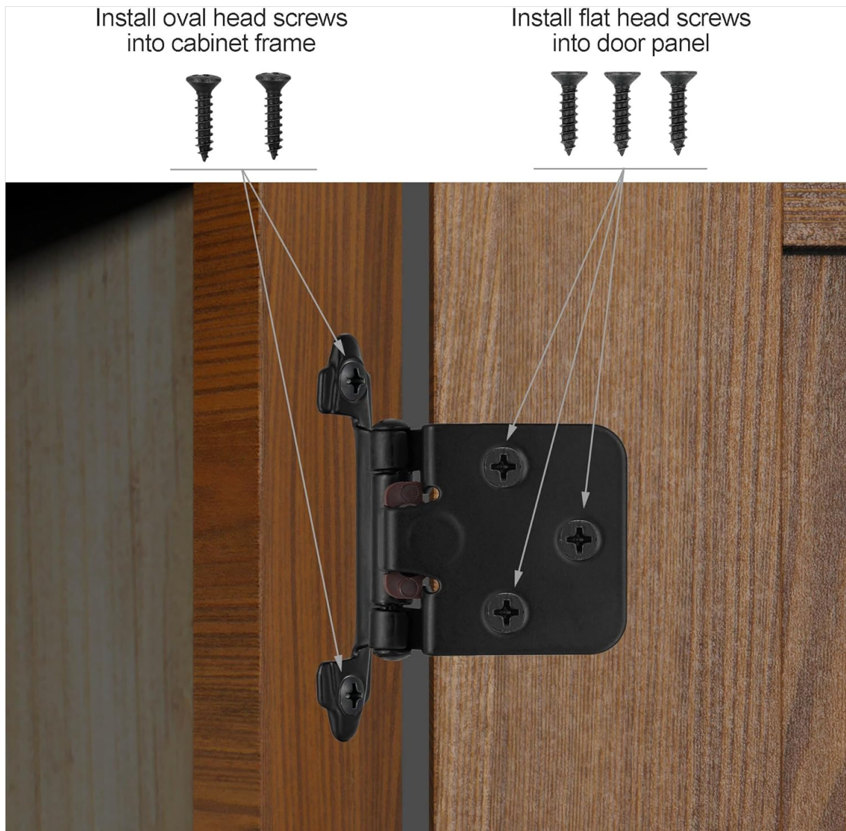
Image: This image demonstrates the correct placement of oval head screws for the cabinet frame and flat head screws for the door panel during hinge installation.
