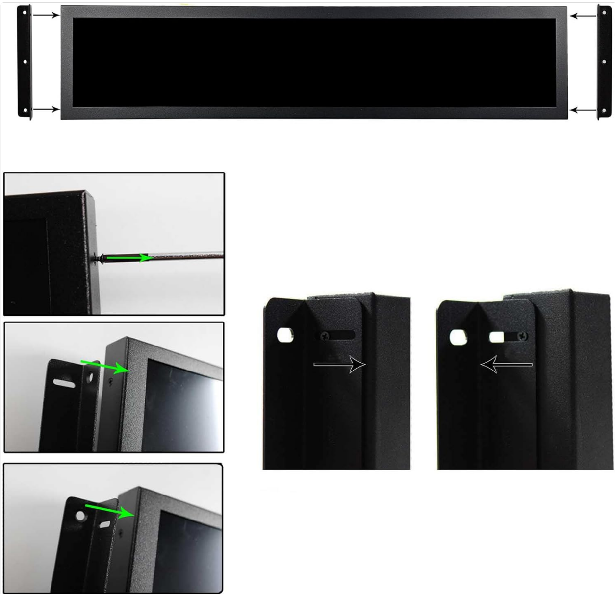
Figure 3.2: Illustration of bracket installation.
